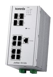
The JetNet 7612G-4F is an pure Gigabit industrial Ethernet Switch with 8 ports RJ-45, 4 ports Gigabit SFP socket for optical fiber network connection. It adopts high efficiency Ethernet MAC controller with 24Gbps Switch fabric bandwidth, 9K jumbo frame forwarding. The robust system design makes the JetNet 7612G-4F survive under harsh outdoor environment with extreme electric magnetic interference and the variation of environment temperature.
