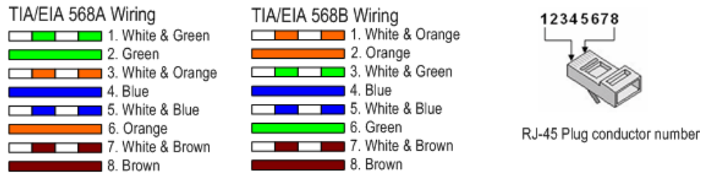
Picture 19 RJ45 Cable color code
