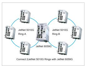
into a line or into multiple directions. In addition to extensibility, MultiRing<sup>TM</sup> has great diversity of various ring technologies. When MultiRing <sup>TM</sup> enabled, JetNet 6059G can connect RSR rings, TrunkRing<sup>TM</sup> and a Super Ring together and simultaneously provide more Gigabit Ethernet Ring connectivity. This provides extensibility to new technologies while keeping the great backward compatibility.
