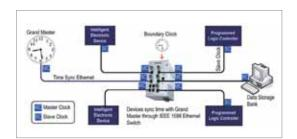
a high level of synchronization within an industrial motion-control environment with a minimum use of network and computing resources. The protocol helps for sequencing event measurements, scheduling outputs, synchronizing actuation, time-stamping, coordinating event records, etc.
