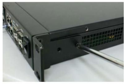
2.10.2 Mount the device in the 19' rack by using four rack-mounting screws provided by the rack manufacturer.
