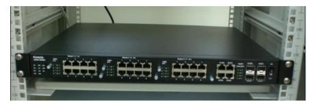
When installing multiple switches, mount them in the rack one below the other. It's requested to **reserve 0.5U-1U free space for multiple switches installing.** This is important to disperse the heat generated by the switch.
