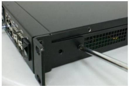
2.2.2 Mount the device in the 19' rack by using four rack-mounting screws provided by the rack manufacturer.
