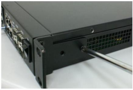
(The picture is JetNet 5628G, the mounting method is the same.) 2.9.2 Mount the device in the 19' rack by using four rack-mounting screws provided by the rack manufacturer.
