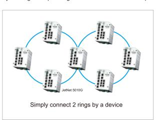
directions. In addition to extensibility, MultiRing<sup>TM</sup> has great diversity of various ring technologies. With MultiRing<sup>TM</sup> enabled, a device can connect RSR<sup>TM</sup> rings, TrunkRing<sup>TM</sup> and a ring of Super Ring together. Which provides extensibility to new technologies while keeping the great backward compatibility.
