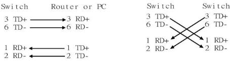
Straight-Through Cabling Schematic
