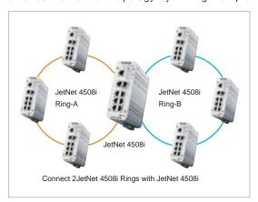
rings into a line or into multiple directions. In addition to extensibility, MultiRing<sup>TM</sup> has great diversity of various ring technologies. When MultiRing<sup>TM</sup> enabled, JetNet 4508i can connect RSR rings, TrunkRing<sup>TM</sup> and a Super Ring together and simultaneously provide more Fast Ethernet Ring connectivities. This provides extensibility to new technologies while keeping the great backward compatibility.
