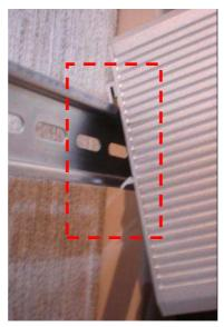
b. Lightly push the bottom of DIN-Rail clip into the track.
