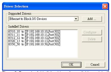
Figure 5: Example: Add all the drivers for available models. If you have 5 models over the same network, add them and give them different name for identification in next steps. Like: (Model Name/6510)\_(IP address/10).
