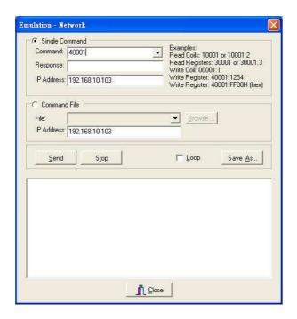
4.1.6.2 Single Command mode. Type the correct IP address of target unit in IP Address field, PLC address in the Command field. Then click "Enter" key. You can read the Response of the PLC address.
