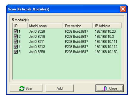
4.1.4.3 Follow the 4.1.4 to practice Jetl/O configuration. Select the model and read or write status and configurations. As to how to operate the Jetl/O configuration of other model, please refer to its manual.
