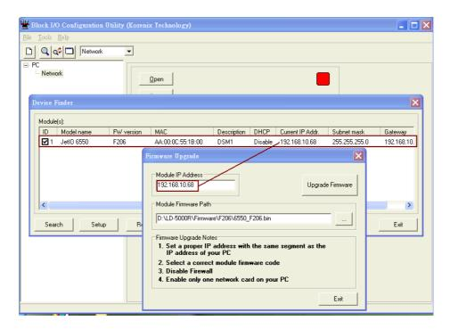
Upgrade Procedure for Mode B (Firmware Resure):
