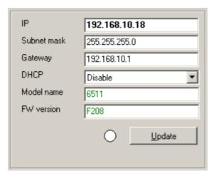
**Note:** After changed IP address or changed the DHCP client mode, the utility will automatically reboot the unit. Please rescan the devices after around 5 seconds.
