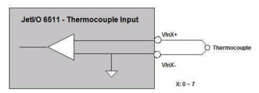
2.4.2 Jetl/O 6511 analog Voltage input wiring example
