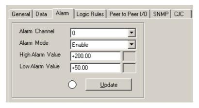
Alarm Channel: Select the channel. Alarm Mode: Enable or Disable
