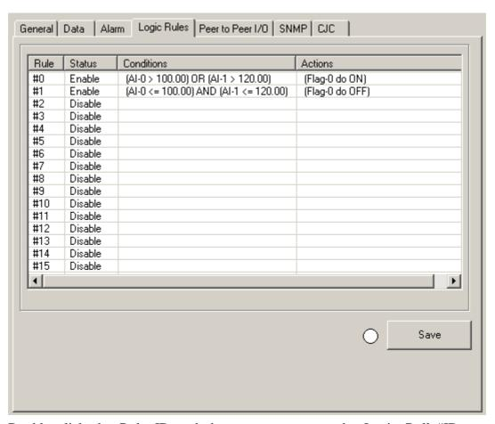
Double click the Rule ID and then you can go to the Logic Rulle#ID Configuration page. Select "Enable" and configure the Condition and Actions then press "Apply" to enable the rule.
