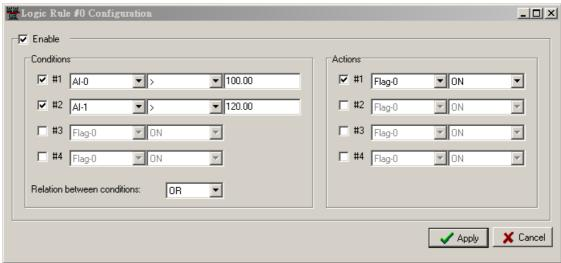
Thus, when the "Conditions" is reached, the system automatically activates the "Actives". For example:
