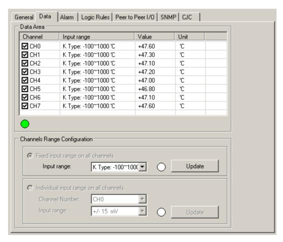
The Channels Range Configuration area, you can choose either "Fixed input range on all channels" or "Individual input range on all channels". The factory default setting is "Fixed input range on all channels". Just select the appropriate range from the "Input range" combo box and then click "Update" to take effect.
