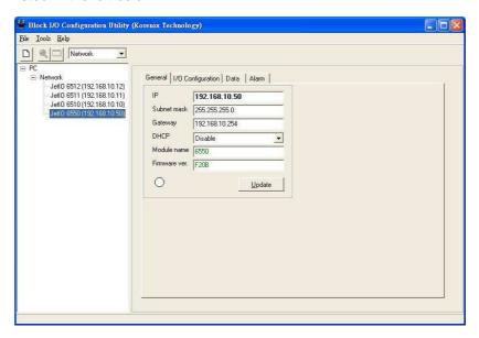
4. Move the mouse over to one of the Jetl/O units. Select the unit then you can configure and monitor the configurations of the Jetl/O. The features Block I/O Configuration utility provides are similar. Please find your model name and go to its configuration introduction chapter in below.
