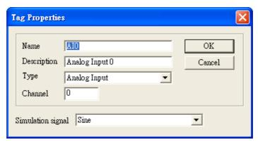
Note: The **Simulation Signal** is used when choosing Simulate I/O mode. Simulate I/O mode is selected in "Device Properties". This feature allows you to generate simulation values and run testing when you operate the OPC client. You can see the value is continuously changed. The Sine, Ramp and Random are the different type's simulation signal.
