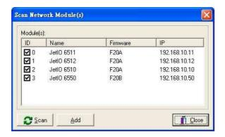
Note: Please modify the IP address of your target devices. The scan feature can't browse the devices which have the same IP address. Only one of the devices which have the same IP address can be found. This is the current restriction. Please modify the IP address first. You can use Block I/O Utility or Device Finder to do the IP modification.
