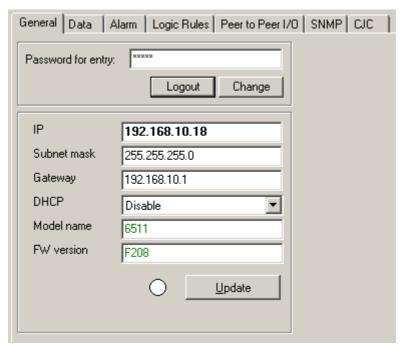
It should be noticed that the privilege setting is required to gain access to do the further configuration options. When you install the I/O module in first time, the default password is "admin". You just need to click on "Login" button and type the password of "Admin" on "password for entry" field. If you want to make password changes, click "Change" button and then the dialog of "Chang Password" prompts you to update the new password with up to six characters.
