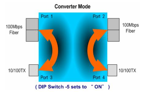
Note: It is necessary to execute system reset or power reset when changing the operating mode; otherwise the new operating setting will not apply.
