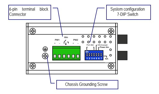
To provide better communication quality and to prevent the interference, it is strongly recommended to make well earth grounding by the "Chassis Earth Ground Screw".
