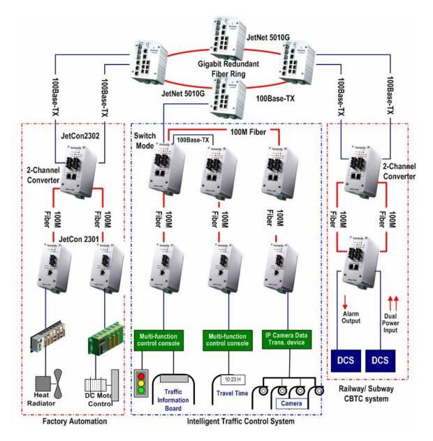
In the application diagram, JetCon 2302 provides graceful anti-electromagnetic interference that ensures the reliable communication not interfered by the noises generated from the motors of facility, railway/subway power system or Intelligent Traffic Control System. The dual channel media converter mode allows reducing the integration cost by simply replacing 2 independent media converters. The switch mode provides flexible connection ability for the network construction.
