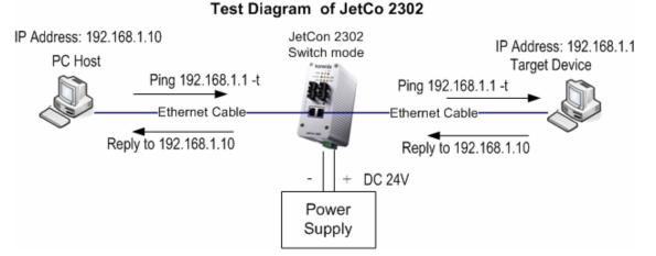
11. Change the mode to converter mode and connect both fiber ports using proper fiber cable, then test the fiber port by sending the ICMP packet process as the procedure-10. The figure of testing architecture is as follows.
