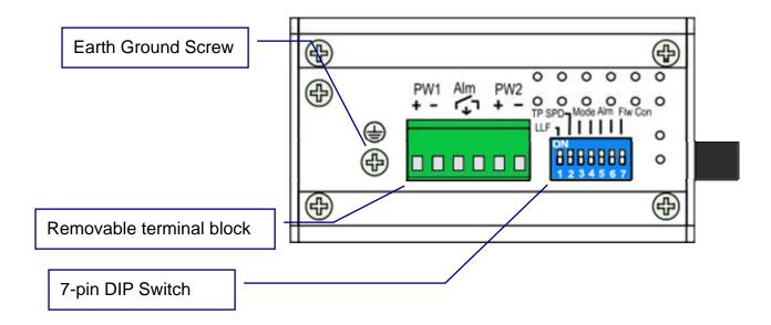
To provide better communication quality and to prevent the interference, it is strongly recommend making well earth grounding by the "Earth Ground Screw".
