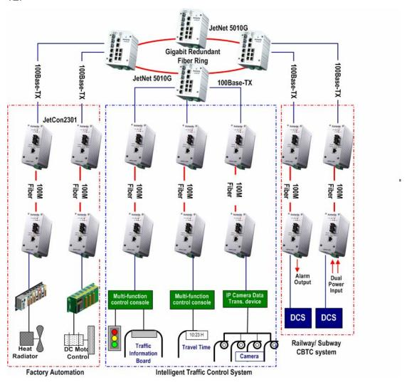
In the application diagram, JetCon 2301 v2 provides signal converting function between upper ring switch and field automation equipments. It delivers 100 Mbps forwarding performance for the extreme heavy loading device which needs direct connection to the backbone, such as the Factory Automation, Intelligent Traffic Control System and CBTC system for Railway/ Subway.
